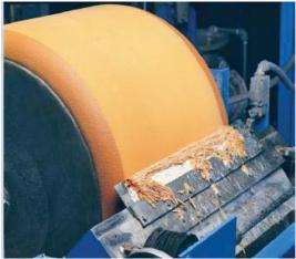
Figure 1: Dry cake being scraped off of a pre-coated filter drum (www.alarcorp.com)
