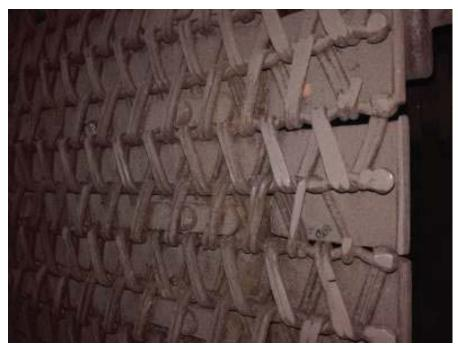
The original diameter of the spirals is 0,16" (4 millimetres); the maximum admitted wear is 30% of the original diameter, so they should measure the diameters in a lot of point of the mesh to be sure that the medium value is more than 0,095" (2,4 millimetres) (measured in vertical direction).
