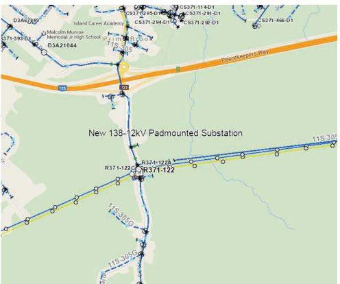
Figure 10 Alternative Sub-D New 138-12kV Pad-Mounted Substation
